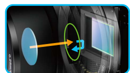
○ Point of focus → Focal plane phase-detection AF → Contrast-detection AF
