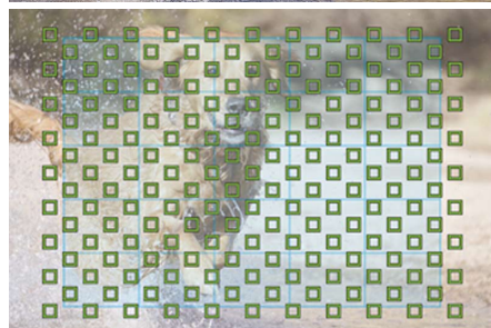
■ Phase-detection AF (179 points) ■ Contrast-detection AF (25 points)
